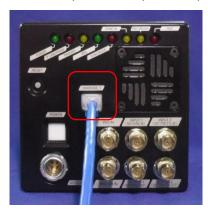
Insert a LAN cable to "1000BASE-T" connector.
